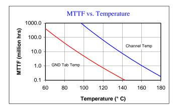
As can be seen from the MTTF numbers above, the predicted failure rate is still above 1 million hours, even at operating temperatures up to  $+115^{\circ}$  C (corresponding to channel temperatures of  $+160^{\circ}$  C). Also note that these MTTF estimates are a lower bound as the accelerated testing never resulted in 50% failures.
